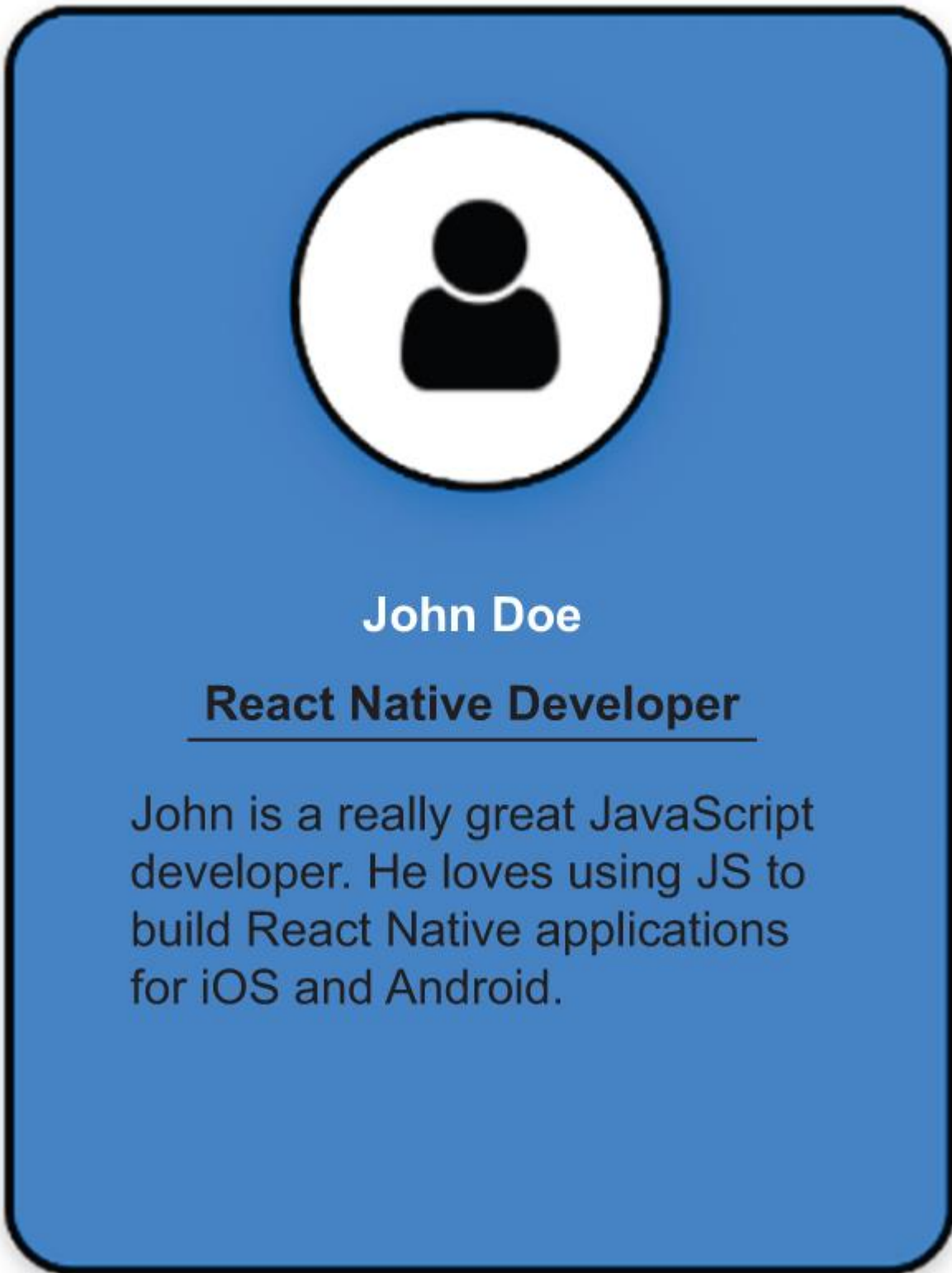
Figure 4.15 The Profile Card with Text elements added using text styling defaults and the color property for the name set to white
