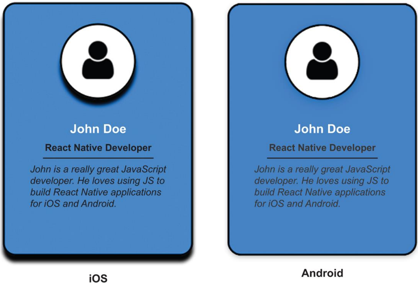
Figure 5.4 The ProfileCard on iOS and Android after drop shadows have been added to the card container and the circular image container. The drop shadows on iOS are created using the iOS-specific shadow properties: shadowColor , shadowOffset , and shadowOpacity . On Android, the elevation property is used to try to create depth. It produces only a minor shadow effect, far inferior to the shadows produced on iOS.
